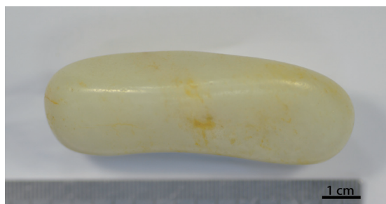
圖2 和田玉仿籽料的打磨面及其交稜 The polished surfaces of Hetian jade pebble imitation and its intersecting edges
