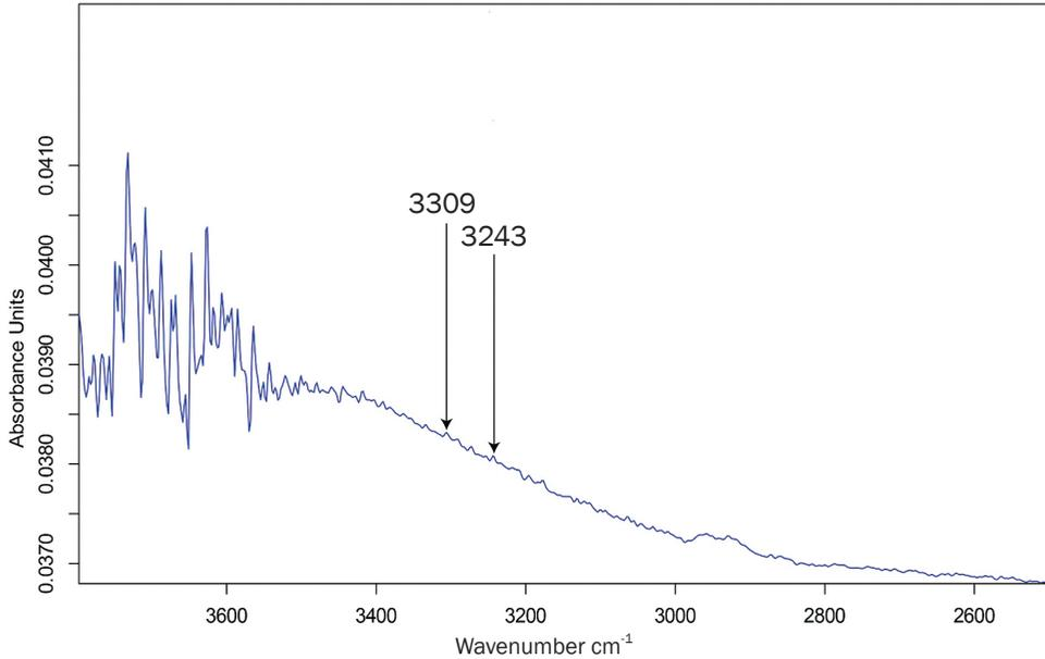
**Fig. 2** Infrared spectrum of a Madagascar pink sapphire using the Pike 4x beam condenser collection attachment. This sends a narrow beam through the gem. Using this technique, the  $3309\text{ cm}^{-1}$  was at the noise floor, while the  $3232\text{ cm}^{-1}$  peak was not visible at all.
