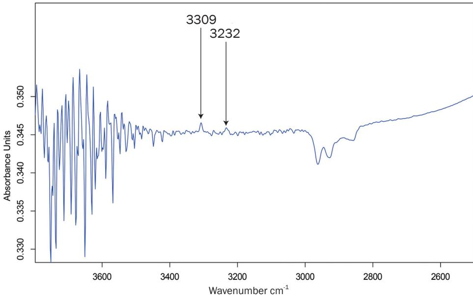
**Fig. 3** Infrared spectrum of the same Madagascar pink sapphire using the DRIFTS (diffuse reflectance) attachment. This bounces the beam through the gem from a variety of directions. Using this technique, the  $3309\text{ cm}^{-1}$  rises well above the noise floor. In addition, the peak at  $3232\text{ cm}^{-1}$  rises above the noise floor, proving that the gem had been subjected to artificial heat treatment.
