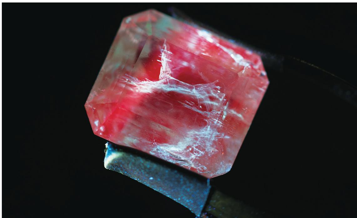
**Fig. 3** When viewed with the Convoy S2+ torch, this Colombian emerald displays a red fluorescence in LWUV. However, the fissure-filling displays a chalky blue reaction because the filler in the fissures (not itself tested and identified) is fluorescing as well.
