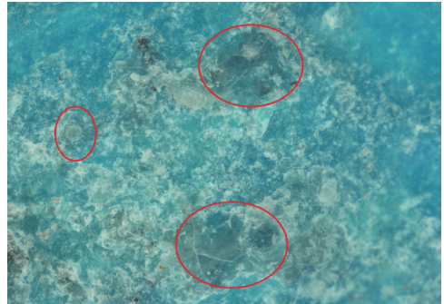
圖3 有機硅充填綠松石原石表面殘留充填物 Surface residue on the organic silicon filled turquoise
