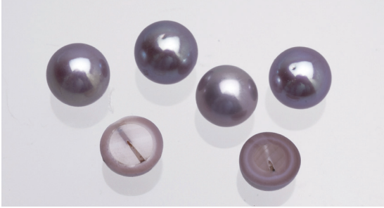
Fig. 3 A group of “Mini Ming” freshwater cultured pearls, the examples that have been cut open display the drilled beads whereas the pearls themselves are not drilled. Diameter of the shell beads is 5mm, thickness of the nacre layer precipitated during 18 months is 1mm. Photo © H.A.Hänni @SSEF
