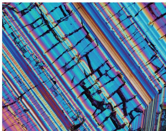
**Fig. 7** Typical zonation in a zircon. The red to orange stripes are richer in U and have therefore expanded more over time. The blue bands are poorer in U and have fractured (the black lines across the bands). Thin section in polarised light, width of image 2 mm.
