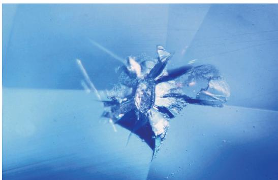
**Fig. 6** A near-surface zircon inclusion in a faceted sapphire from Sri Lanka. Volume increase due to radioactive self-bombardment has increased the volume size of the crystal, causing pressure on the host sapphire. As the crystal is very near to the surface, it has blown away a part of the overlaying sapphire. Magn. 15X.
