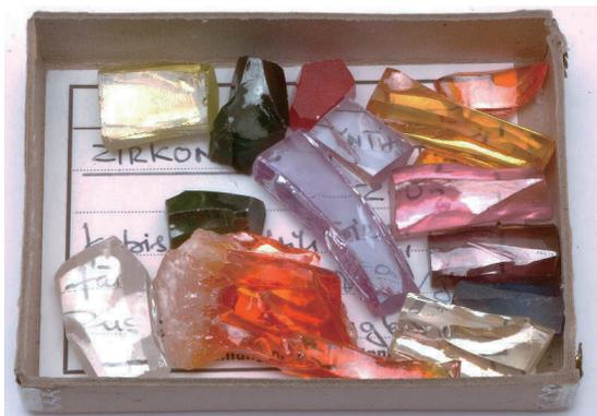
**Fig. 11** A collection of broken pieces of zirconia rough. The coloured pieces are doped with REE's. The box is 5 cm long.
