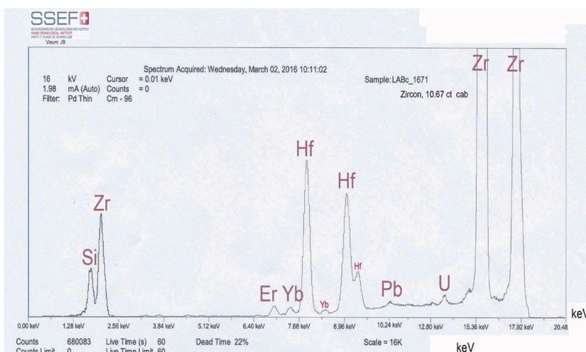
**Fig. 3** Qualitative ED-XRF analysis of the metamict zircon from Tanzania in Fig. 8. Main constituents Si, Zr, REEs (Rare Earth Elements) Er, Yb, and Hf show up, as well as heavy elements U, Pb.
