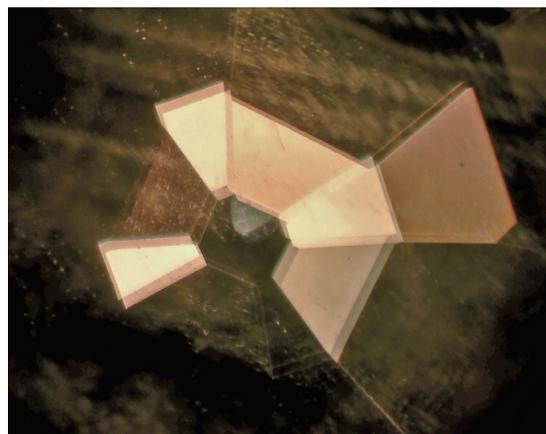
**Fig. 4** A faceted octagonal step cut zircon of 24.5 cts. The back facets are visible twice. The doubling is due to the orientation of the stone (maximum double refraction perpendicular to the optical axis). Magn. 10X.
