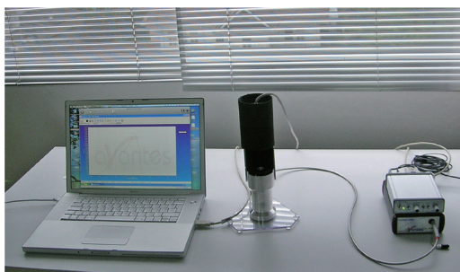
Fig. 9 Portable UV-Vis spectrometer developed by the SSEF Swiss Gemmological Institute. This instrument uses a small spectrometer, which can simply be plugged into a laptop. © M.S. Krzemnicki, SSEF 2008
