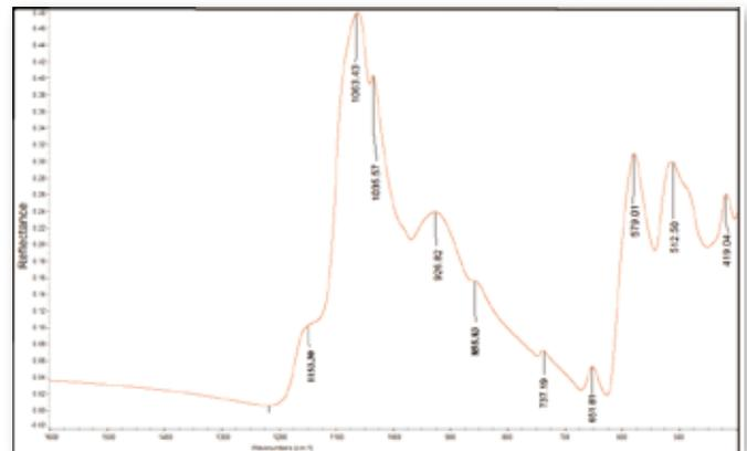
Figure C: Typical Specular reflectance FTIR fingerprint spectrum of Fei Cui, Kosmochlor Jade.
