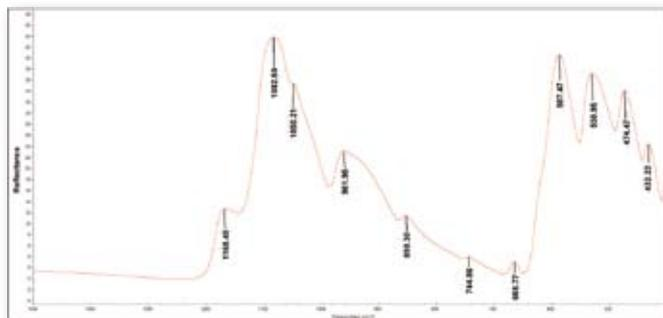
Figure A: Typical Specular reflectance FTIR fingerprint spectrum of Fei Cui, Jadeite Jade.
