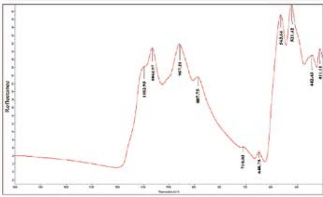
Figure B: Typical Specular reflectance FTIR fingerprint spectrum of Fei Cui, Omphacite Jade.
