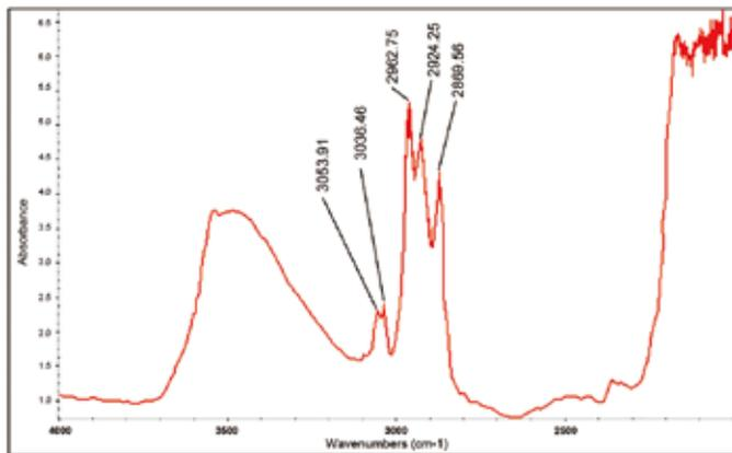
Figure A: Spectrum of a typical resin impregnated Fei Cui using transmittance method.
