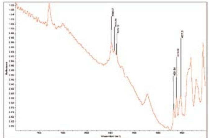
Figure B: Specular reflectance FTIR spectrum of a typical resin impregnated Fei Cui, showing groups of peaks at around  $5900\text{ cm}^{-1}$  or  $4680\text{ cm}^{-1}$ .
